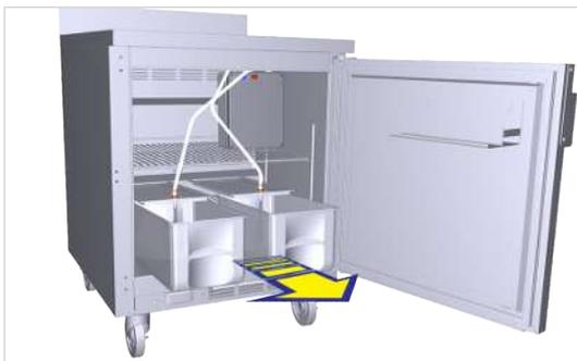
3. Pull out the milk container and remove the container lid.
