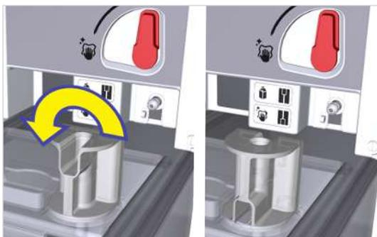
3. Pull the reversible adapter upwards and from the suction fitting.
