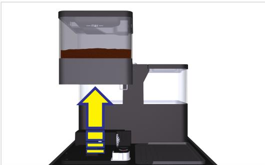
2. Lift and remove the powder hopper.
