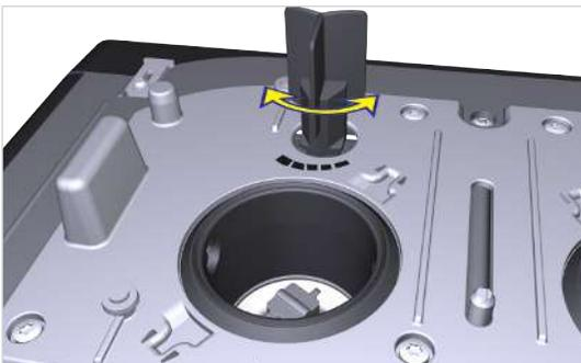
3. If necessary, adjust the grind coarseness using the grinder adjustment wrench.
