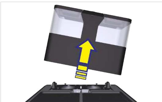
2. Remove the bean hopper by lifting it upwards.
