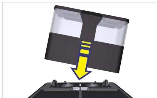
7. Attach the bean hopper and powder hopper (if applicable).
