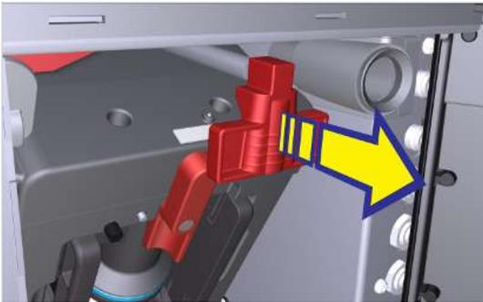
1. Pull the locking slide towards the front up to the stop.
