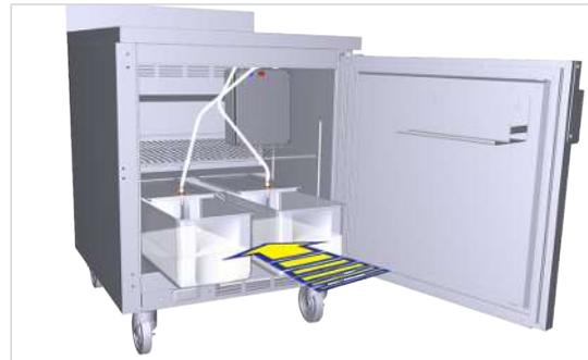
5. Slide the milk container into the refrigerator.
