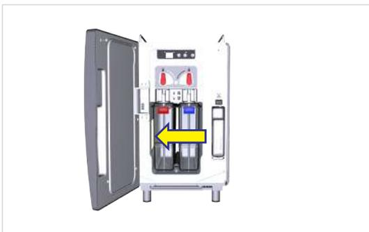
The type plate for the cooling unit is located on the left-hand side in the cooling chamber.
