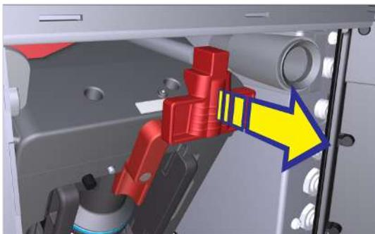
2. Pull the locking slide towards the front up to the stop.
