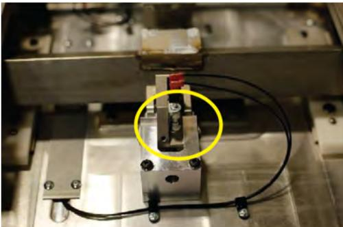
4. Manually lift the upper pressure pin until the microswitch changes position.
