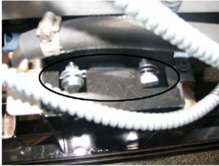
12. Install the two screws connecting the filter pump to the face of the filter motor.
