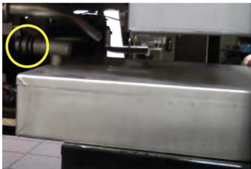
4. Inspect the three o-rings at the rear of the reservoir and replace o-rings that are missing, excessively worn, or damaged.
