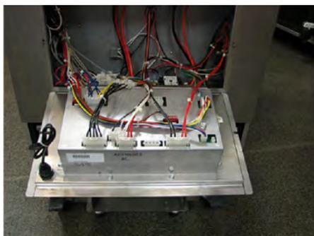
3. Disconnect all the connectors on the back of the control board.
