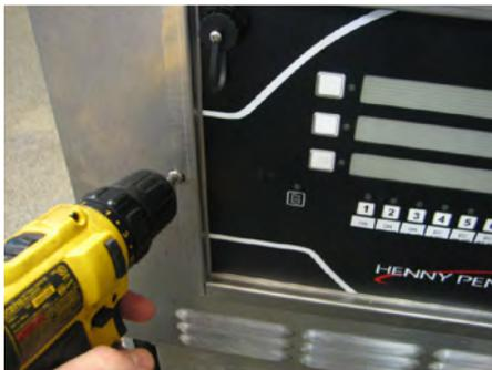
1. Use the Phillips head screwdriver to remove the two screws securing the control board to the front shroud.
