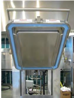
1. Lift the lid, tilt back and lock in to place.
