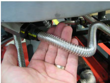
1. Notice the routing of the old flex tube before removal.
