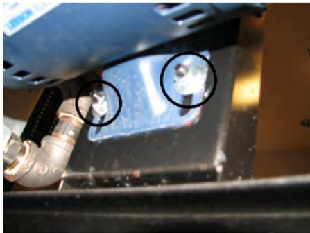
3. Use a Phillips head screwdriver to remove the two screws that secure the plate onto the pump motor.
