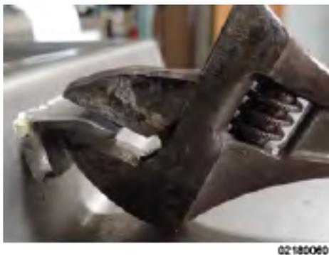
4. Adjust the catch with an adjustable wrench. Gently flex the catch up or down as required.
