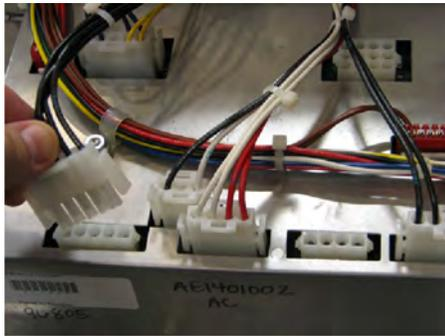
6. Place new control board on to the unit with the tab inserted in to the slot. Let the control board rest on the shroud.
