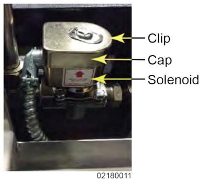
22. Reinstall the coil over the bonnet with the conduit on the left side so it does not interfere with the lid cables.
