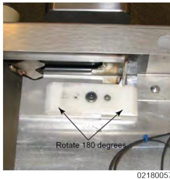
3. If any excessive wear is found, the pad will need to be rotated by removing both screws and rotating the pad 180°.
