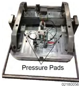
1. If necessary, push the lid cam back off of the pressure pads.
