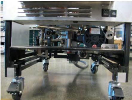
1. Remove the drain pan, fresh oil pan (ATO), and condensation pan.
