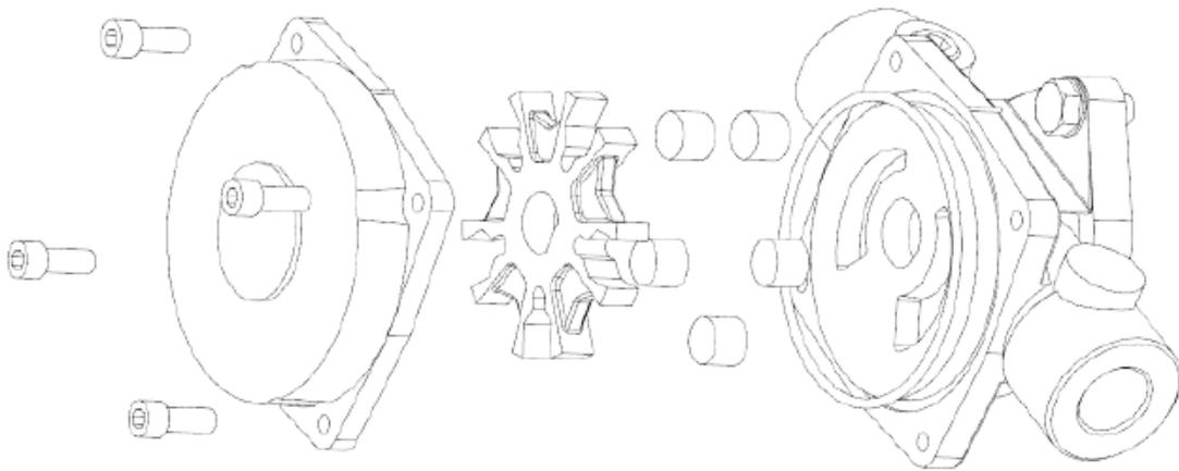
Figure 5-2 Pump Rollers
