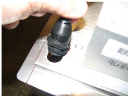
4. Disconnect the USB plug from the receiver on the back of the control board.
