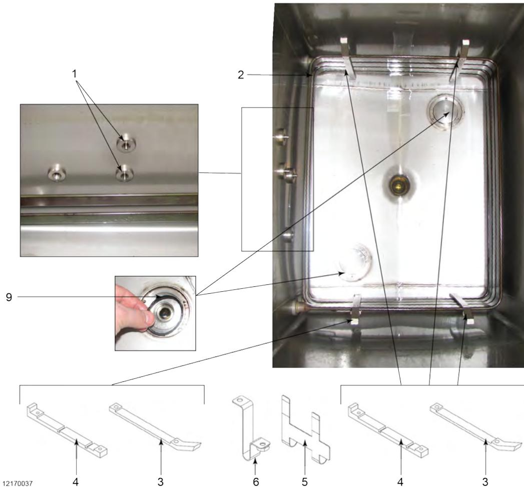
**Figure 6-3 Heating Element**
