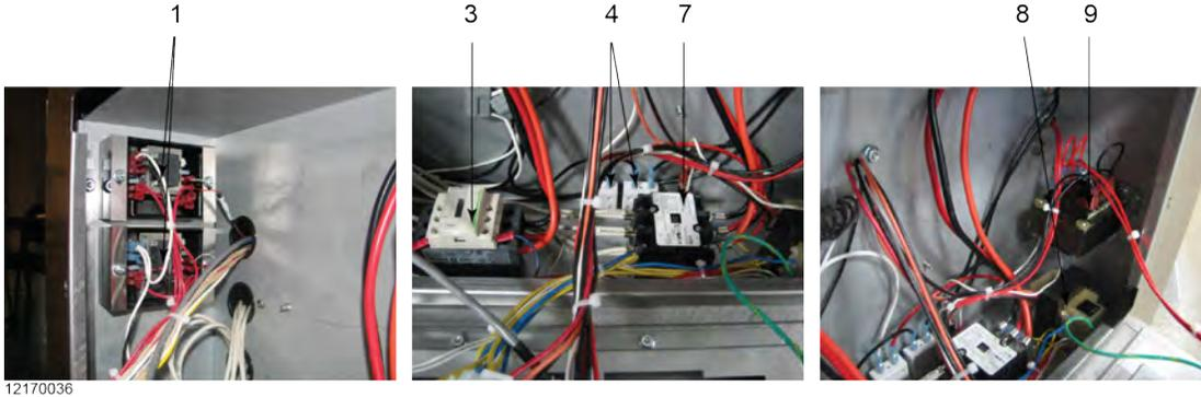
**Figure 6-4 Thermocouple, Heat Contactor & Control Transformer**
