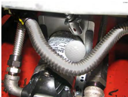
3. Use the old flex tube as a template to rough bend the new tube.
