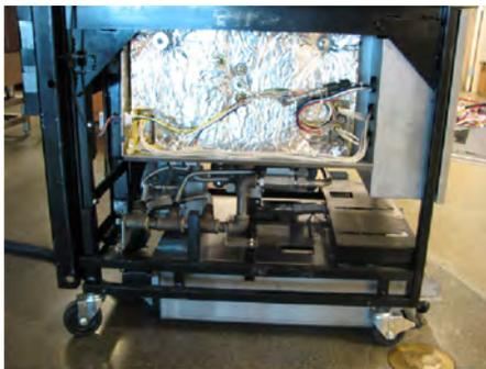
3. Use a Phillips head bit to remove the screws from the left-hand (from the front of the unit) side panel.
