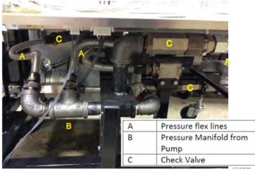
1. Use a flashlight to inspect the fittings of the filtration plumbing and between the filter pump and motor for oil leaks.
