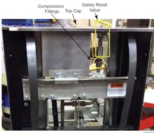
1. If necessary, remove the steam exhaust, top cap cover and 6 keps nuts around exterior of rear cover, and then remove the back shroud of the fryer.
