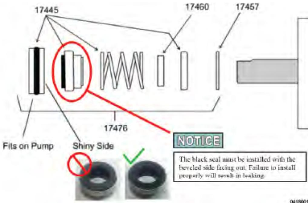
Figure 5-1 Pump Seal Kit Placement
