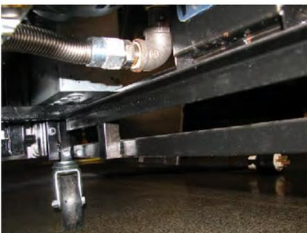
2. Use an adjustable wrench to remove the flex line and pipe connections from both ends of the pump motor.
