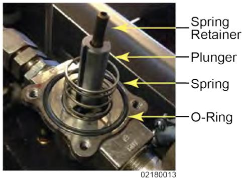
17. Install the o-ring into the valve body's o-ring groove.
