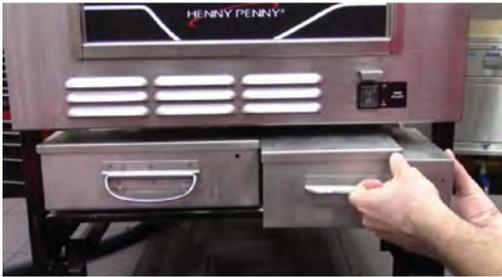
1. Remove the condensation drain pan to the right of the ATO reservoir.
