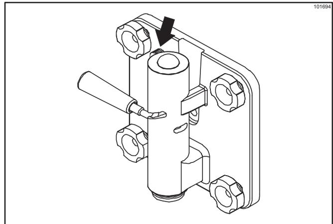
5. Place the mix hopper cover in position. For proper operation, there must be a substantial amount of mix in the hopper. If the ADD MIX light illuminates, refill the mix hopper as soon as possible.
